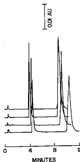
Figure 1. Dial-a-Mix technique using on-line mixing of 55% bottle A (0.1 M acetate) and 45% bottle B (methanol). The first peak is testosterone, the second is corticosterone.
