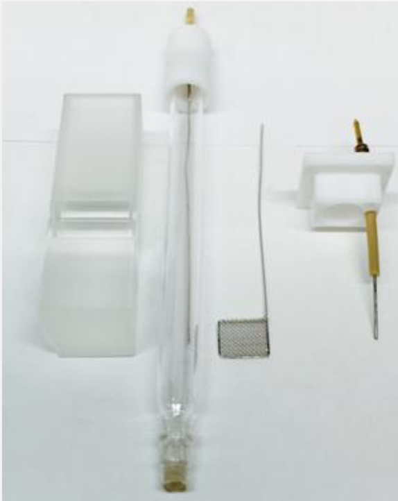
Figure 3. Components of a UV-vis SEC cell.
