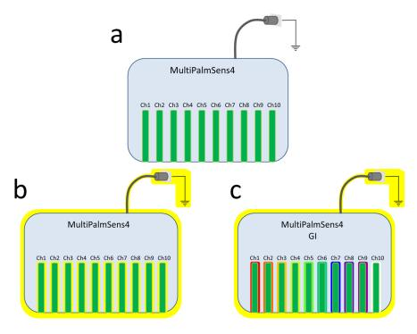
Figure 2.1 a) Scheme of a MultiPalmSens4 with its PCBs; b) MultiPalmSens4 with yellow halo indicating the same ground; c)
